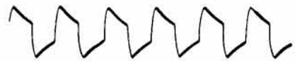
2. Square wave distortion from poor response at both high and low frequencies.
