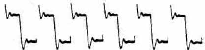
3. Square wave test on feedback amplifier showing peak at 9 times square wave frequency.
